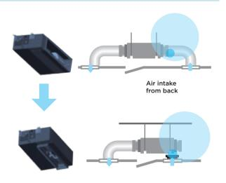
Whether return air is required from the rear or bottom, both can be easily achieved on-site by changing over the cover, as both air inlet have the same frame size.
